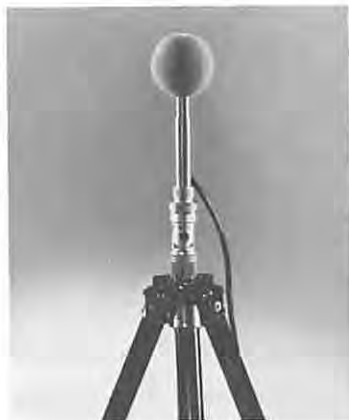
Figure 6-15. A typical field installation for microphone use. The tripod mount is shown supporting a Type 1560-P42 Preamplifier, into which a 1/2-inch microphone has been plugged. The foam sphere at the top is a windscreen that fits over the microphone to permit accurate measurements outdoors.
