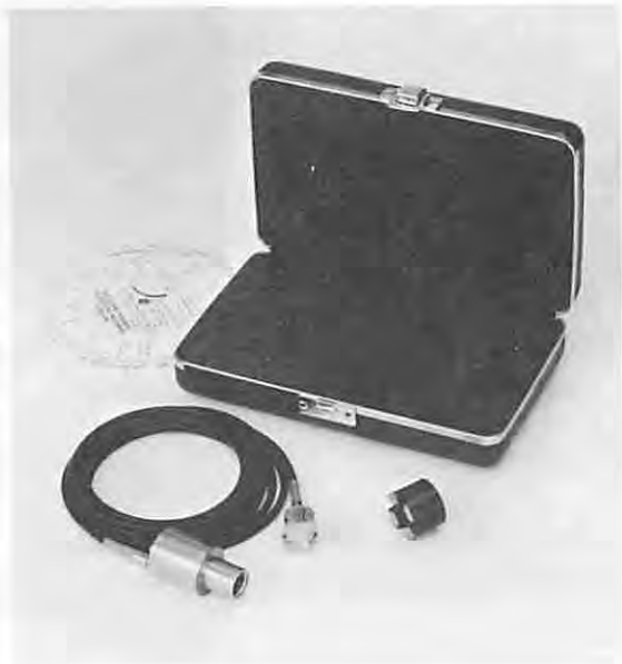
Figure 6-19. Vibration integrator system.
