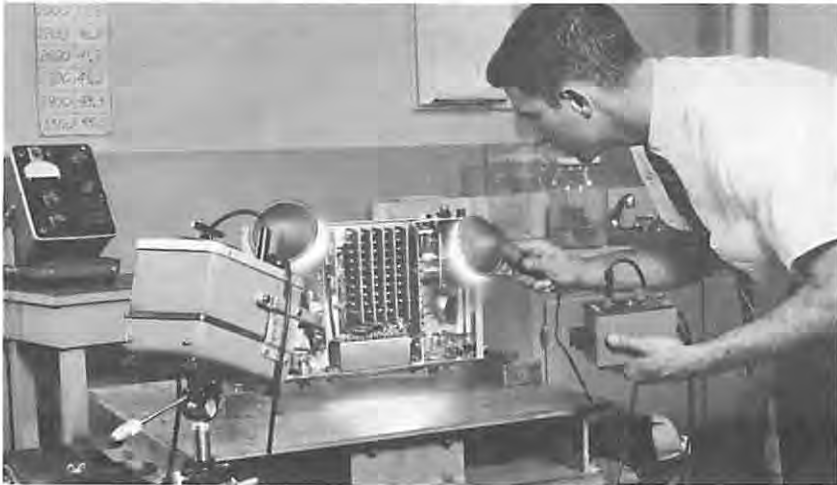
Figure 10-8. Combination of instrumentation forces to solve a vibration problem. Shown are the Types 1538 and 1539 Stroboscopes to study the motion of parts on an electronic assembly being exercised on a shake table.
