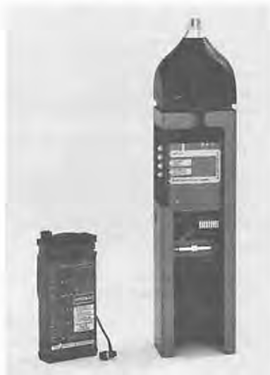
Figure 3-1. The GR 1954 Noise Dosimeter. The monitor on the left can be clipped in a shirt pocket or on a belt. The indicator on the right is used to read out the accumulated noise dose at the end of the measurement period.
