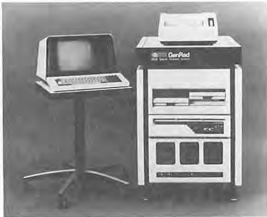
Figure 9-6. The GR 2505 Signal Analysis System for analysis of one or two-channel data by FFT processes.
