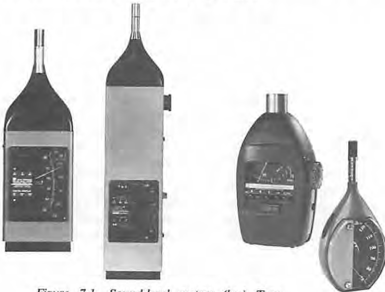
Figure 7-1. Sound-level meters (l.r.) Type 1981-B Precision (ANSI Type S1A), Type 1982 Precision SLM and Analyzer (ANSI Type 1), Type 1565-B (ANSI Type 2), Type 1983 (ANSI Type S2A).
