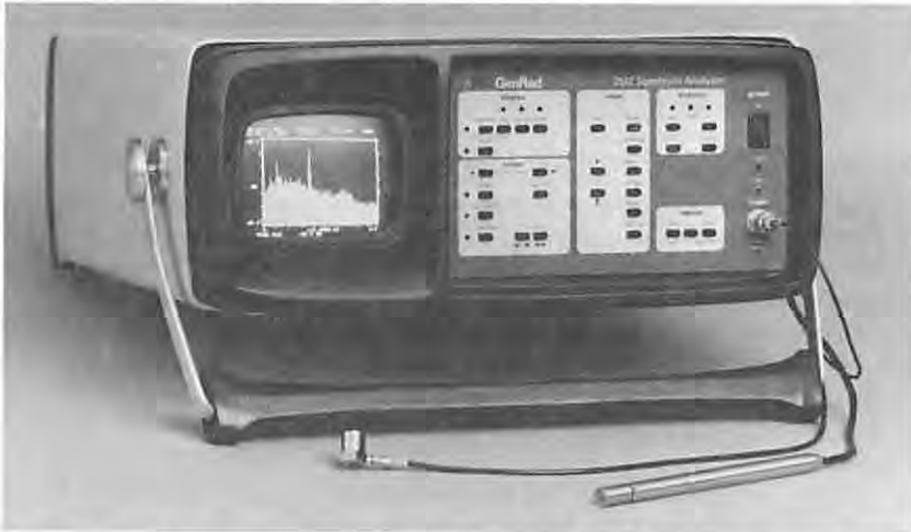
Figure 9-5. A high speed spectrum analyzer that uses a fast Fourier transform to provide 400 lines of resolution.
