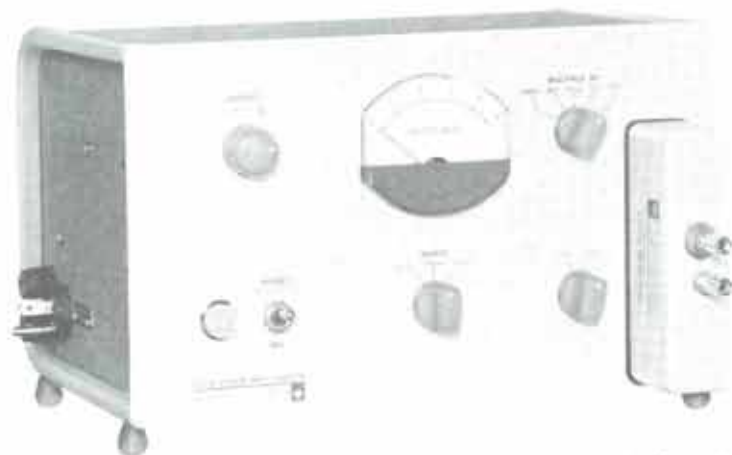
Random-Noise Generator with Pink-Noise Filter plugged in.
