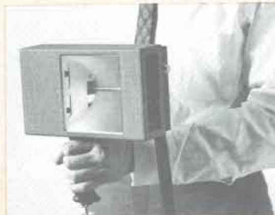
The lamp-head assembly can also be hand-held separately using the pistol-grip handle supplied.
