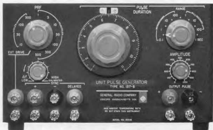
Figure 1. Panel view of the Unit Pulse Generator.
