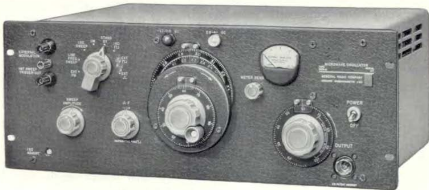
Figure 1. Panel view of the Microwave Oscillator.
