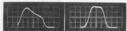
▼ Figure 9. I-F response of television receiver, as measured with direct output of sweep oscillator (available at rear of generator). Left-hand curve was taken before adjustment, right-hand curve after adjustment for best characteristic. Frequency at center line is 44.5 Mc.
