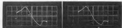
▲ Figure 8. Aural discriminator characteristics of television receiver, under slightly differing conditions of adjustment. Center frequency is 4.5 Mc; scale 50 kc/cm.
