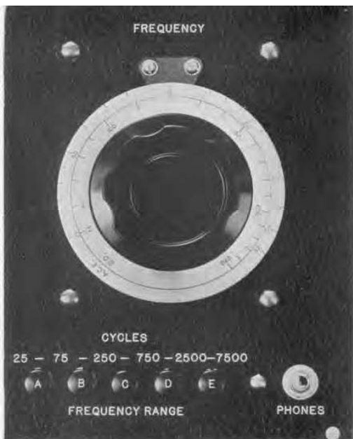
FIGURE 3. The tuning controls consist of a single dial and a row of push-button switches. The dial frequency span in cycles per second for each range is engraved above the corresponding push button, i.e., 25-75, 75-250, etc.
