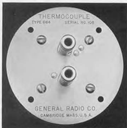
FIGURE 1. Front view of the TYPE 664-A Thermocouple showing the standard-voltage terminals. The circular plate mounts in the shield or on the panel of an r-f generator.
