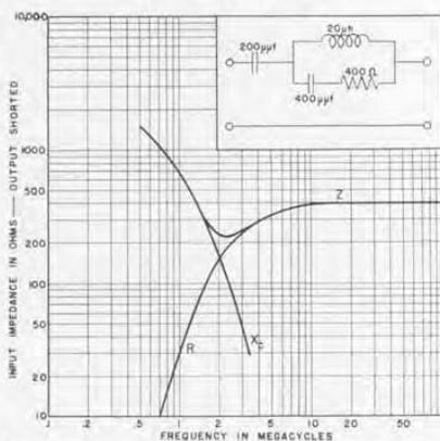
FIGURE 1. Resistance, reactance, and impedance characteristics of the TYPE 418-G Dummy Antenna
