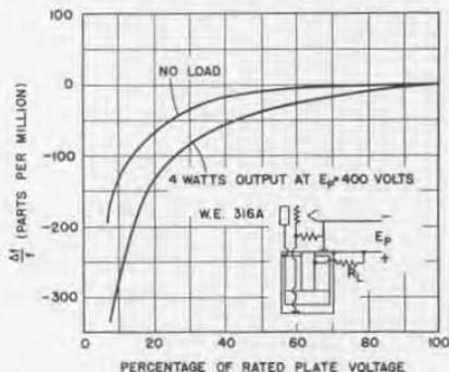
FIGURE 4. Change in frequency produced by a variation in applied plate voltage. The upper curve is taken at no load, the lower with a load of 4 watts
