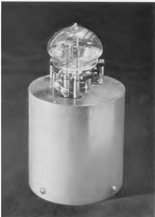
FIGURE 1. The complete oscillator consisting of tank circuit and vacuum tube. The over-all height is 7 inches
