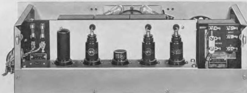
FIGURE 3. Rear view of the power-level indicator with dust cover removed. Note that all tubes are easily accessible from the rear
