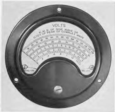
FIGURE 5. Five ranges of voltage are provided. It will be seen that the scales are nearly linear
