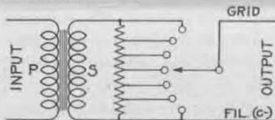
Such a potentiometer is likewise useful as a voltage divider to increase the range of a vacuum tube voltmeter and in numerous other lines of research.
